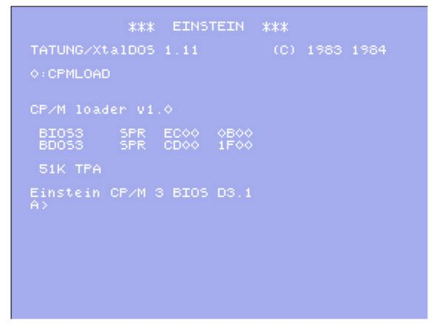
The CP/M+ operating system for the Einstein was developed by Duncan Elvin some years ago. It does not require its own boot disk but loads on top of Xtal DOS.
