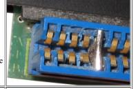
Although there was continuity between the individual contacts and the corresponding PCB terminals, many of the contacts had a noticeable lack of "spring".
