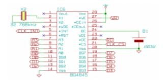
The interrupt line is the real reason I included it though. It has internal facilities to generate an interrupt periodically (once per second, minute, hour etc. up to month) using the alarm, or more frequent interrupts, from just over 30uS to half a second, using the periodic, counter interrupt. This attracted me to the device, as there is no internal counter in the Z80 and I have grown accustomed to writing multi-tasking systems that jump to another task on a timer based interrupt.
