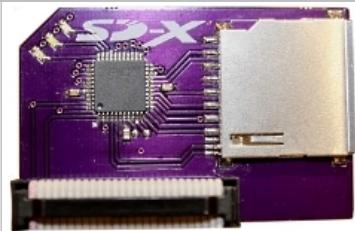
The SD-X board is connected to the Einstein "Pipe" interface connector - a 60 pin IDC socket on the rear of the computer case.
