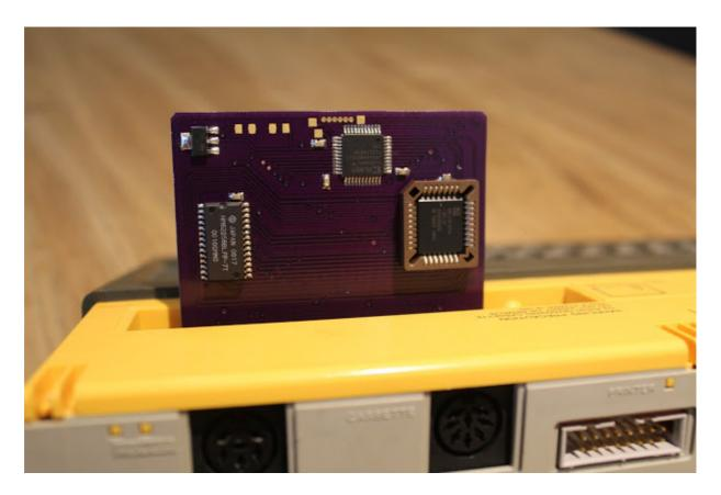
I just need to adjust the size of the printing on the front and move a capacitor so that the EEPROM socket doesn't foul on it but other than that I believe it's good to go!
