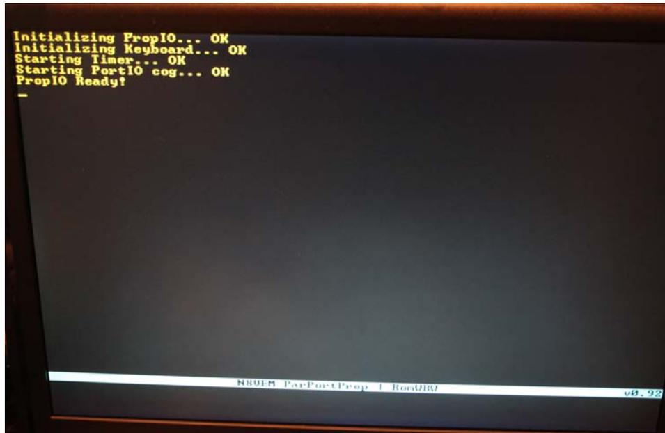
9. The last step is to place both the N8VEM CPU and the PropIO in the backplane sockets and power up the pair with CPU JP2 removed. The VGA will run
