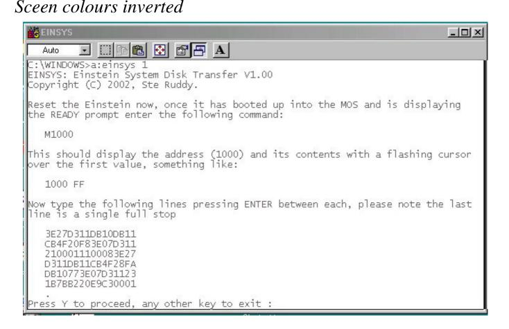
On the Einstein type "M1000 <ENTER>" as instructed then the lines of hexadecimal digits using <ENTER> at each lines end. After typing the full stop on the last line press the <ENTER> key to end the modify command and return to MOS. At the MOS prompt type "G1000 <ENTER>.
