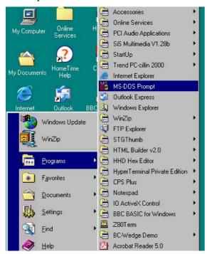
On the PC windows desktop double click for the MS-DOS Prompt to get the DOS window. By typing "C:\WINDOWS>a:einsys 1" at the dos prompt to use com1 serial connection or "a:einsys 2" to use com2 then <ENTER> will start einsys running displaying instructions and the Hex that has to be typed into Einstein.
